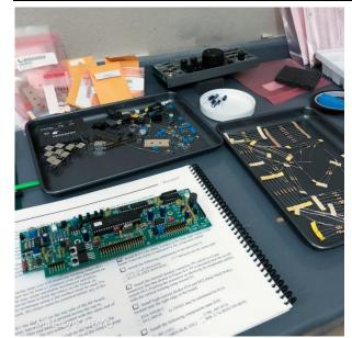
The second phase of the assembly is all on the RF board, and it starts with resistors—lots of resistors. I use small baking pans, an ice cube tray, upside down lids, and a small hobby bin to keep things organized. To speed installation, I taped all the remaining electronic components on to a piece paper in the order that they appear in the manual.
