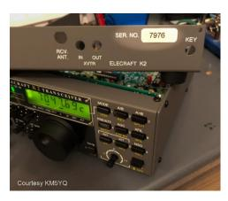
I spent some more time aligning the 4 MHz reference oscillator using my KX3 as a source. I had a small wire "antenna" connected to the K2, basically 7 inches of wire with a loop at the end that came with my KX3. Interestingly, I actually received a S5 or 6 high-speed CW signals on that little piece of wire around 7.040! Wow!
