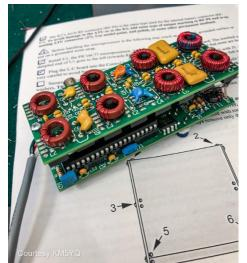
Now, that I had the basic K2 completed and aligned it was time to finish building the automatic antenna tuner (ATU). There were two boards to complete: a Control board and an L-C board. The L-C board was a little challenging as most of the .001 pF caps and relays were installed on one side, and the large caps and inductors were installed on the other side of the board. The challenging part of the build here was that the leads for the large caps and inductors had to be
