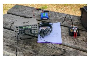
I found a covered picnic table at Cedar Hill State Park around 2:00 pm in the afternoon and setup my Buddipole<sup>TM</sup> as a 20m vertical. The vertical section was a full size ½-wave—no coil needed—along with a wire counterpoise running down one of the guy lines. The ATU quickly brought the SWR from 2:1 down to a 1.0:1 match after a few seconds of clicking relays.
