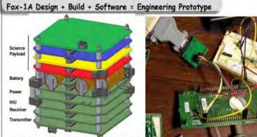
Fox-1 Stack: 400 mW TX downlink on 2M, 70 cm RX, IHU with 32-bit processor, 128K program memory, 16K RAM, 128K MRAM to store telemetry and experiment data.
